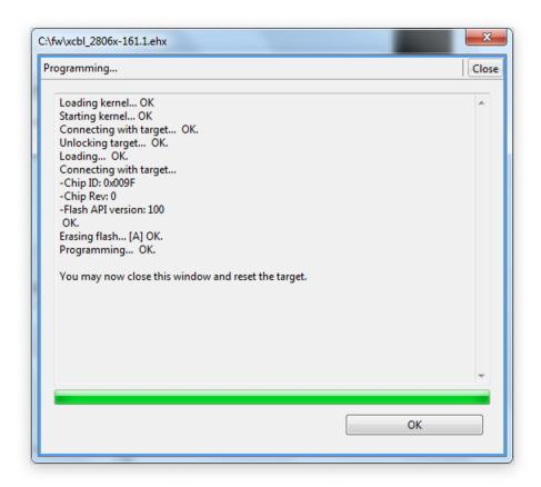
Finally, you may save the programming configuration combined with the firmware image to an Extended Hex file by clicking the **Save as ehx...** button. When this file is subsequently selected in C2Prog, all programming settings are automatically configured. This format is therefore recommended for distributing firmware images.
